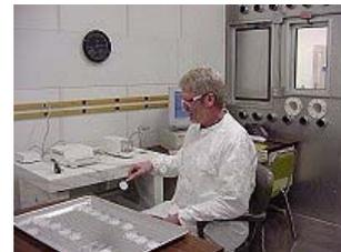
Filter being weighed at the ORIA Montgomery, AL laboratory to determine particulate matter.
