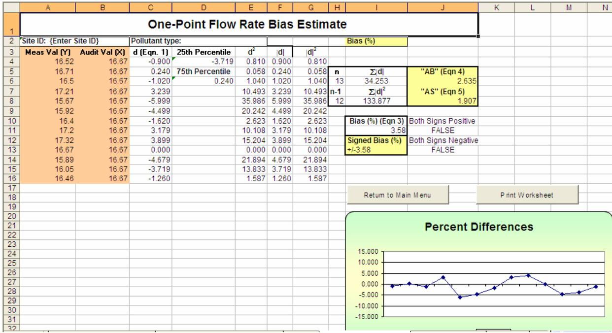
Figure 10. One-point flow rate DASC worksheet example
