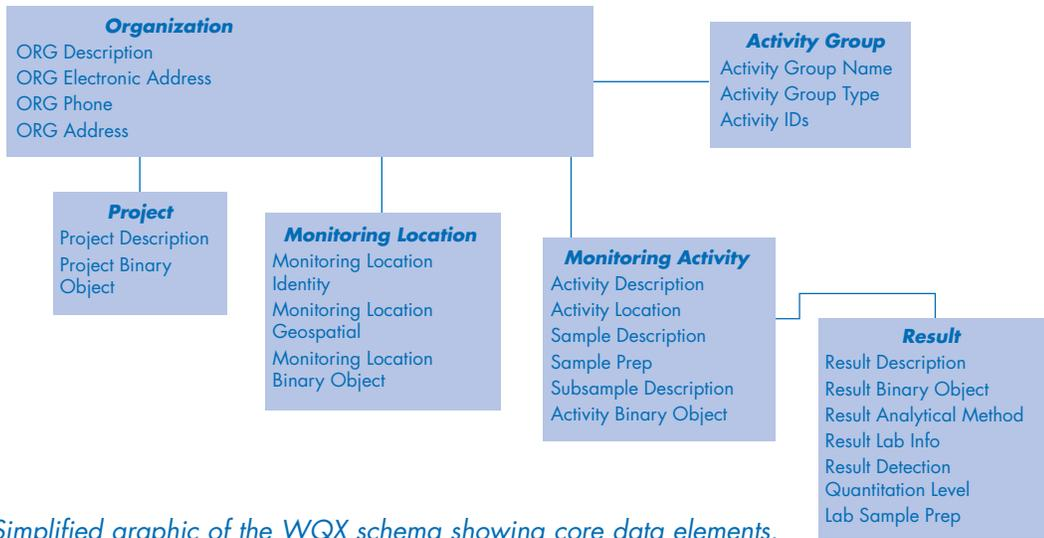
*Simplified graphic of the WQX schema showing core data elements.*
