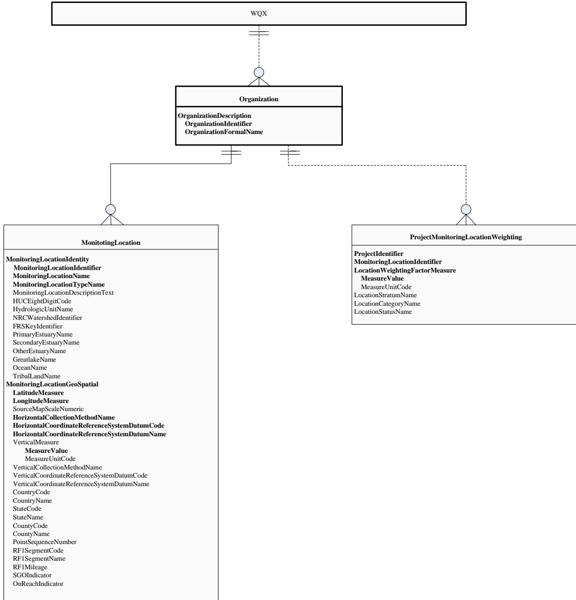
Figure 8.2 —Station Web Service Output Schema - getStationInfo
