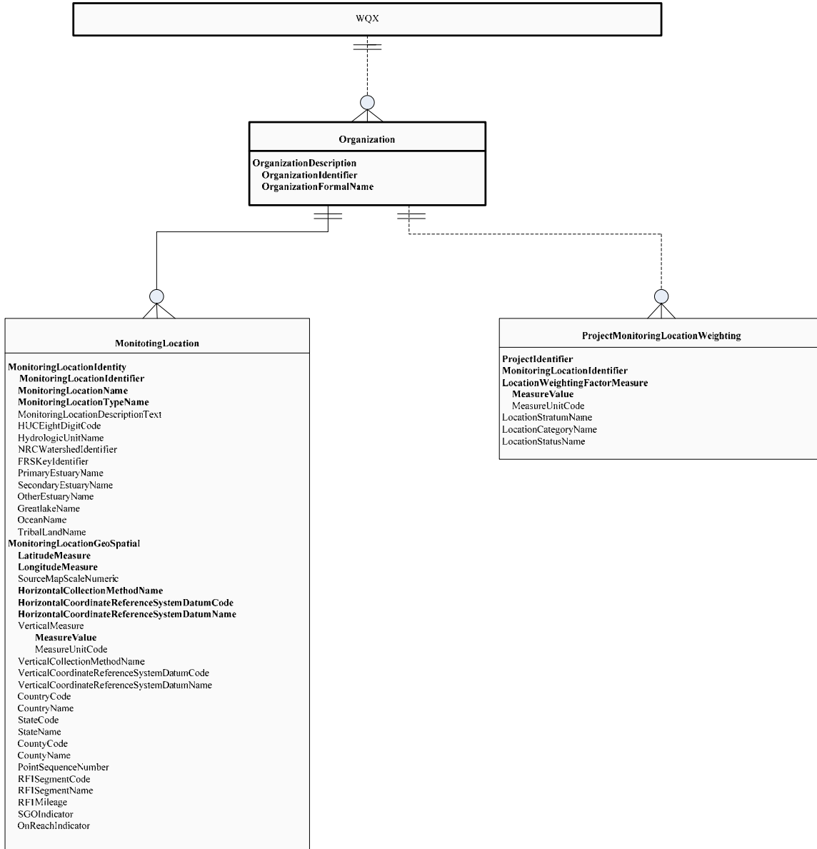
Figure 8.2 —Station Web Service Output Schema - getStationInfo
