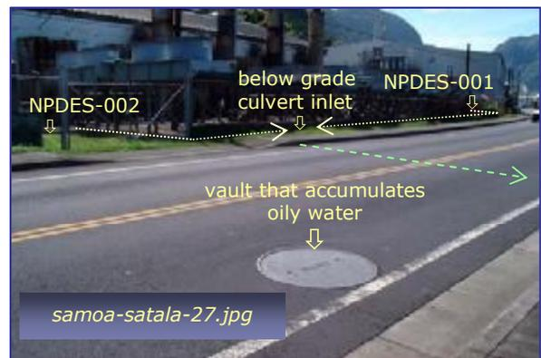
Photo #6: Power Plant and Vault Location
