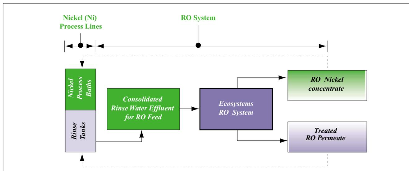
**Figure 4. RO System Schematic at Perfection Plating**
