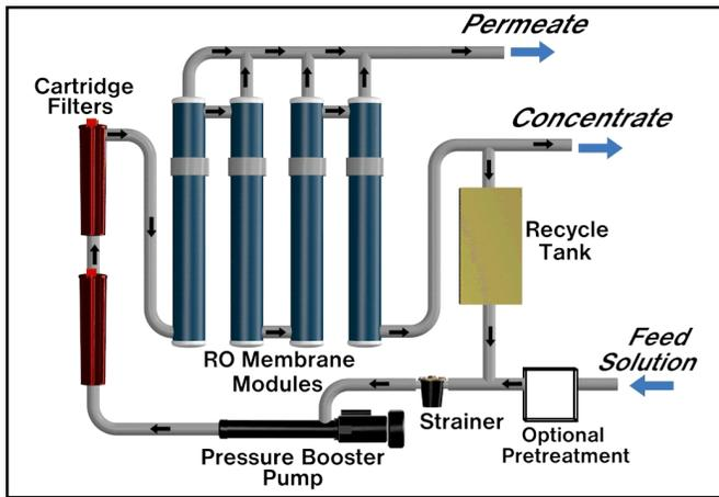
**Figure 2. Basic Components of an RO Unit**
