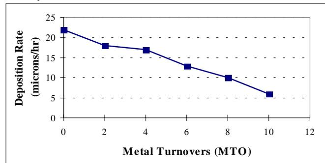
**Figure 1. The EN deposition rate decreases by 40 percent after six MTOs. In most commercial applications, EN baths average five MTOs for aluminum parts and seven MTOs for ferrous parts before they are spent.**
