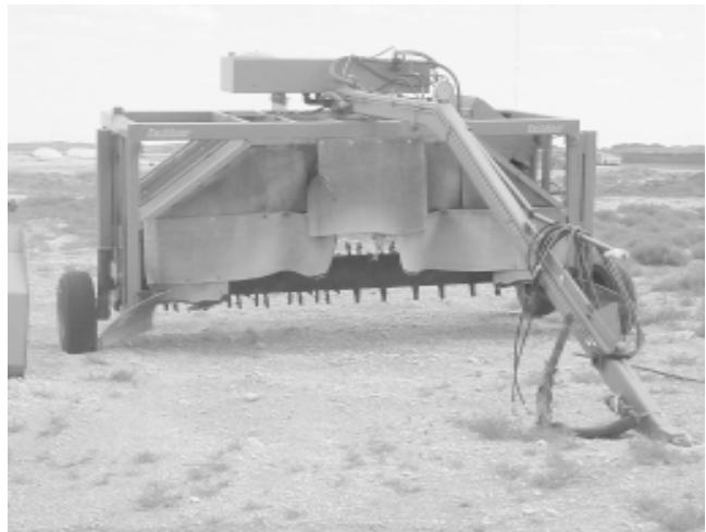
Figure 2. When temperatures fall below 145°F, the pile can be turned using a windrow turner.
