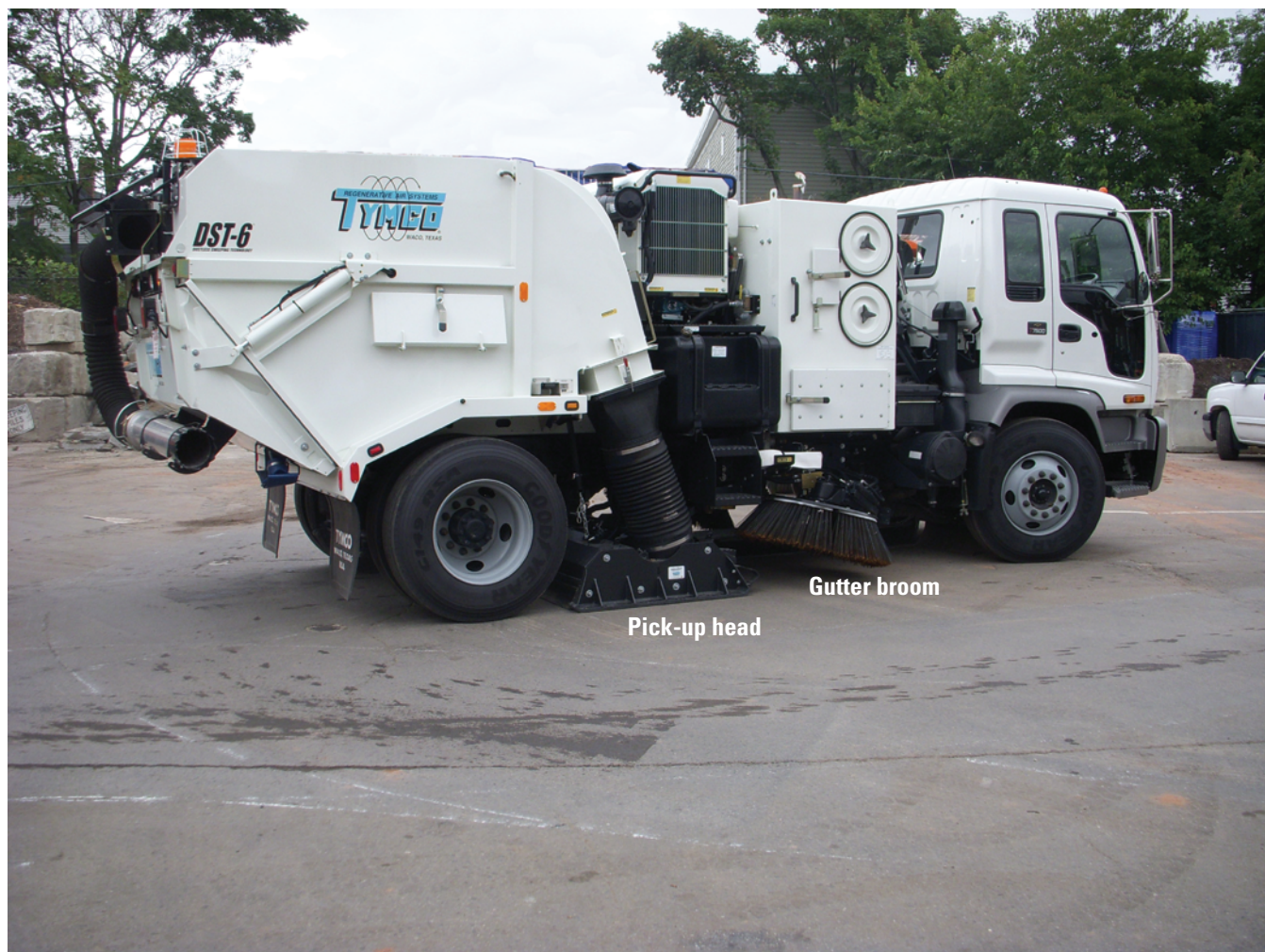
Figure 6. Photograph of a TYMCO Dustless Sweeping Technology-6 (DST-6) regenerative-air street cleaner in Cambridge, Massachusetts (photo courtesy of Tom Maguire, MassDEP).
