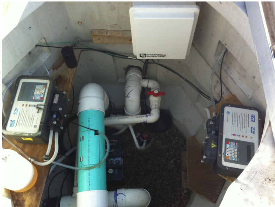
Figure 2. Monitoring equipment and elevated outlet pipe, modified bioretention, Storrs, CT.
