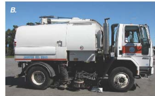
Figure 4. A, Pelican Series P mechanical sweeper and B, Johnston 605 Series vacuum sweeper, used in the evaluation of sweeper efficiencies.
