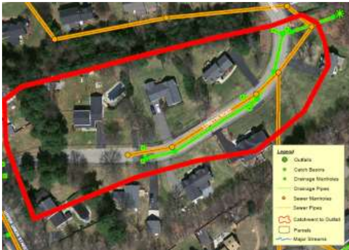
Figure 1. The final permit requires permittees to map outfalls (green asterisk in upper right corner); drainage areas or catchments to each outfall (in red); associated storm drain inlets and pipe network (in green); sewer lines (in orange); and associated manholes like those shown here from a catchment in Franklin, MA. Geographic Information Systems (GIS) can be a valuable tool for gathering, depicting and analyzing MS4 mapping data.
