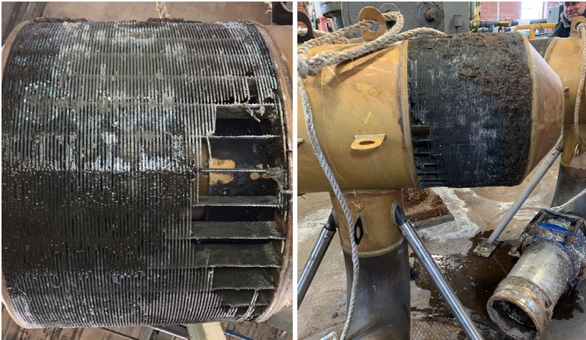
Figure 3. Imagery of damaged portions of the test wedgewire screen assembly.
