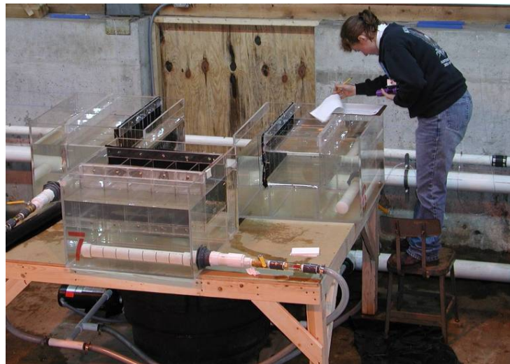
Figure 7-9 Biological testing facility comprised of 14 small acrylic test flumes (EPRI 2004)
