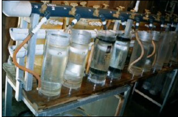
Figure 7-6 Hatching jars used in American shad egg impingement trials at the New York State Department of Environmental Conservation (NYSDEC) (photo courtesy Ed Radle, NYSDEC).
