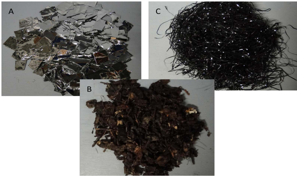
Figure 2-42 The surrogate debris group included mylar (A), wood chips (B), and tinsel (C) debris
