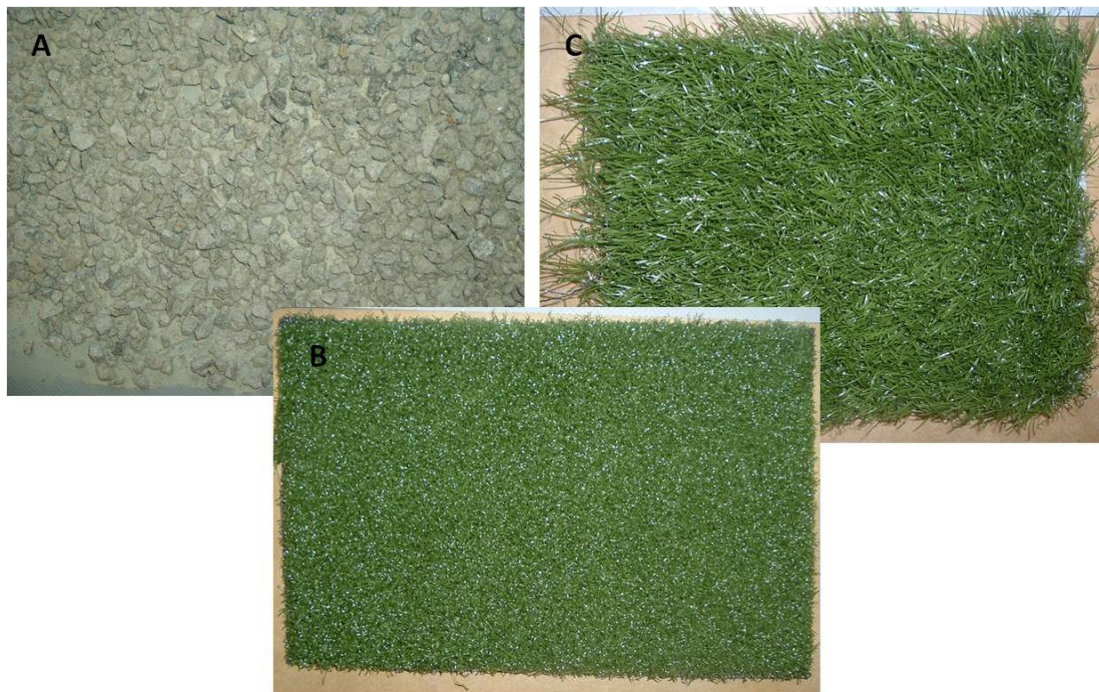
Figure 2-40 Stone (A), rough carpet (B), fiber (C) and smooth (not shown) trough substrate materials
