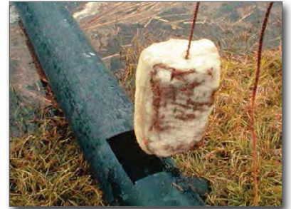
Figure 19. Polymer blocks inserted into pipes
