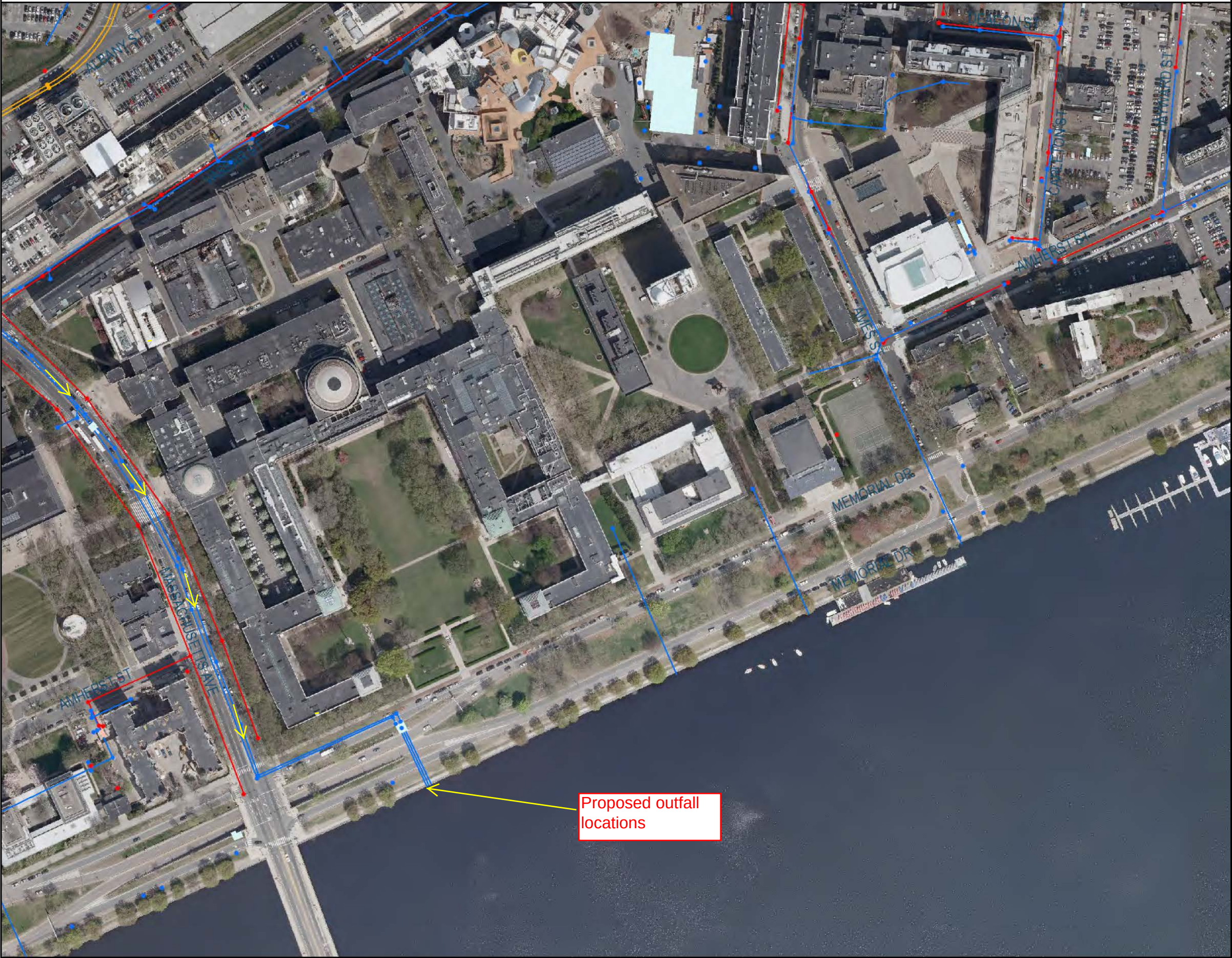
FIGURE 5 - PROPOSED DEWATERING DISCHARGE ROUTE
