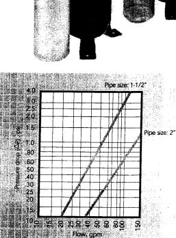
Based on housing only. Fluid viscosity, filter bag used, and expected dirt loading should be considered when sizing a filter.
