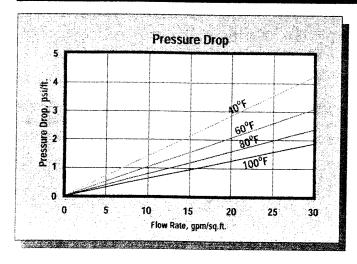
PRESSURE DROP - The graph above shows the expected pressure loss per foot of bed depth as a function of flow rate, at various temperatures.
