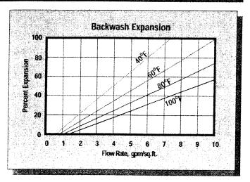
BACKWASH - After each cycle the resin bed should be backwashed at a rate that expands the bed 50 to 75 percent. This will remove any foreign matter and reclassify the bed. The graph above shows the expansion characteristics of RESINTECH CGS in the sodium form.
