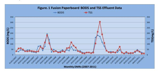
The proposed effluent limitations for  $BOD_5$  and TSS are an average monthly limit of 300 mg/l and a maximum daily limit 490 mg/l, respectively, which are in the range of typical untreated domestic sewage (medium to strong concentrations). These proposed effluent limitations for  $BOD_5$  and TSS are considered to be protective of the City of Norwich WPCF operations.
