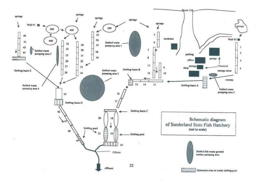
Attachment B. Schematic Diagram of Sunderland Fish Hatchery
