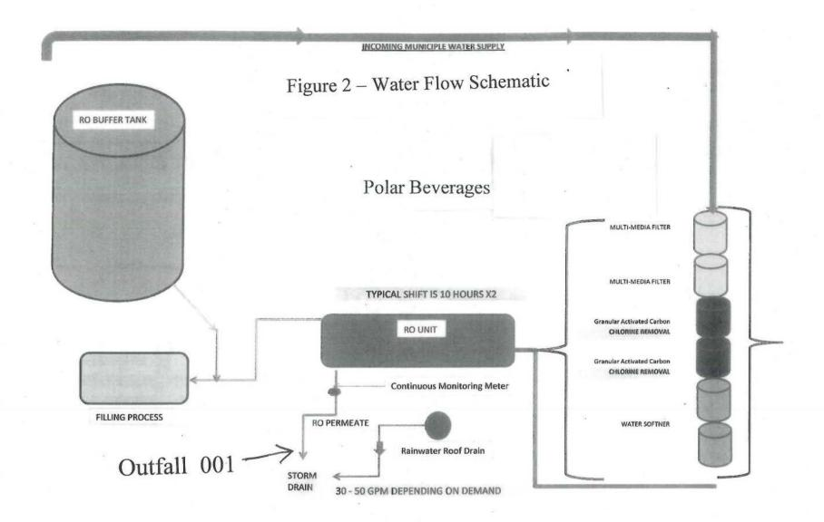
Plan for RO permeate water is to pipe a continuously monitored discharge pipe to an existing roof drain that discharges directly to the storm water drain.
