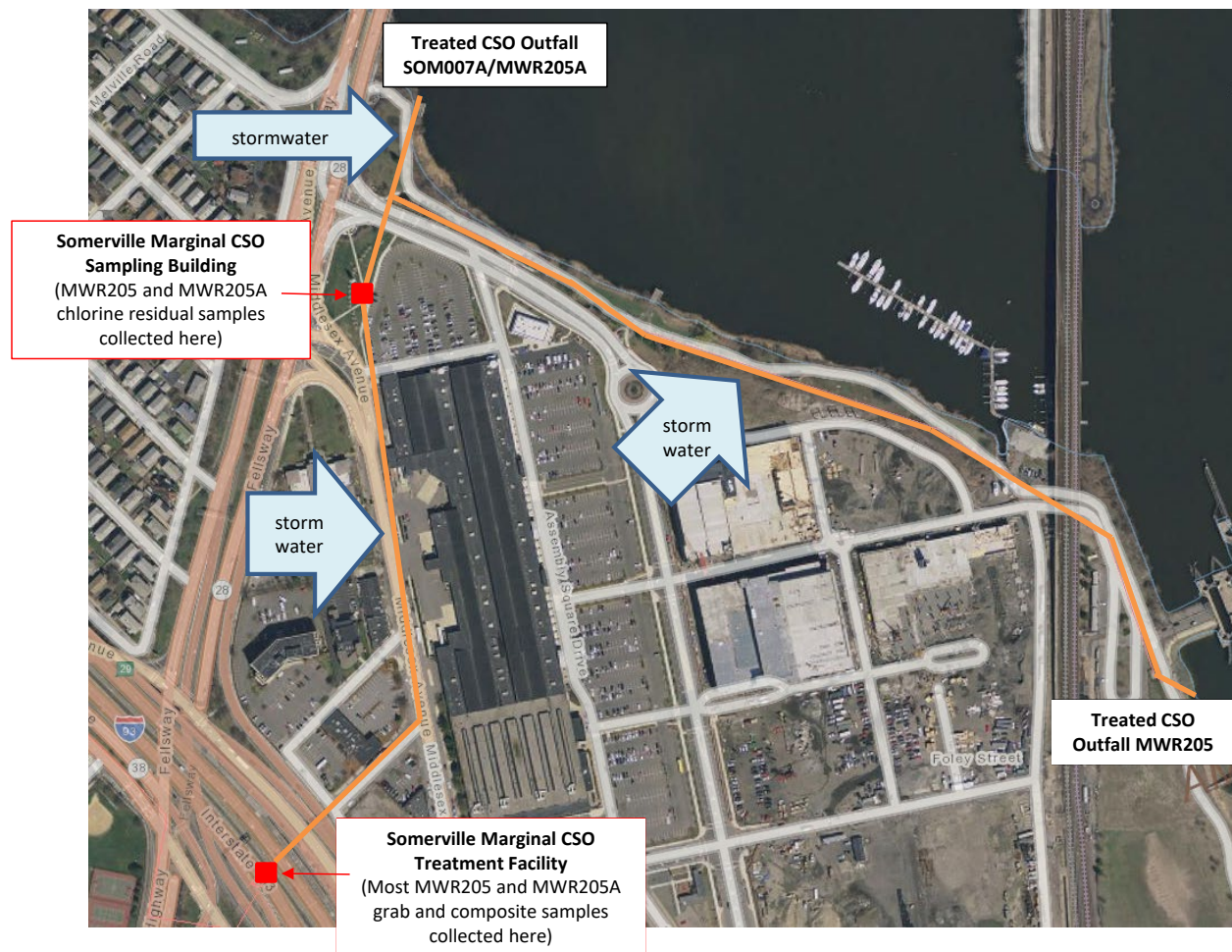
Figure 1. Diagram showing the Somerville Marginal CSO Treatment Facility and outfalls MWR205 and SOM007A/MWR205A.
