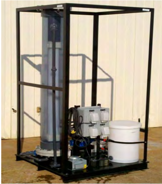
Figure 5. Membrane Operation System (MOS) Pilot Unit using POREFLON Membrane.
