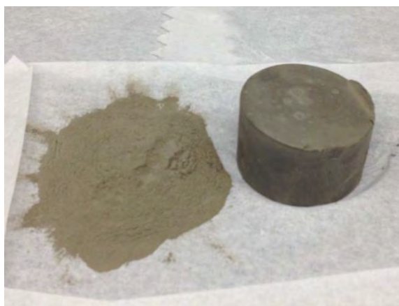
Figure 2. Picture of S/S solid. Coal fly ash is shown on the left.
