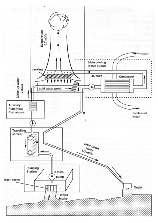
Figure 1: Schematic representation of an open recirculating system. (Jenner et al 1998)<sup>13</sup>
