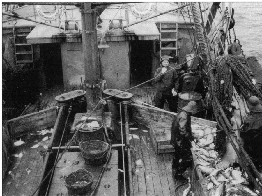
Figure 3. A side-trawler capturing Atlantic cod off the coast of Nova Scotia on La Have Bank in the early 1950s. One of the two large doors of the otter trawl is seen suspended next to the vessel and is used to spread the net as it is towed along the ocean bottom. Trawlers have remained an important component of the overall fishing fleet in the northwest Atlantic.
