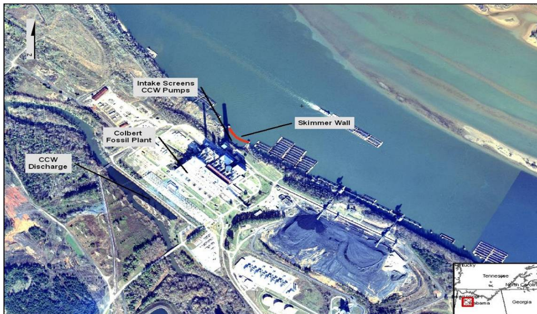
Figure 24-1 Aerial Photograph of Colbert Fossil Plant Cooling Water Intake Depicting the Skimmer wall, Condenser Cooling Water Pumps, Intake Screens and Discharge Channel in Northwest Alabama
