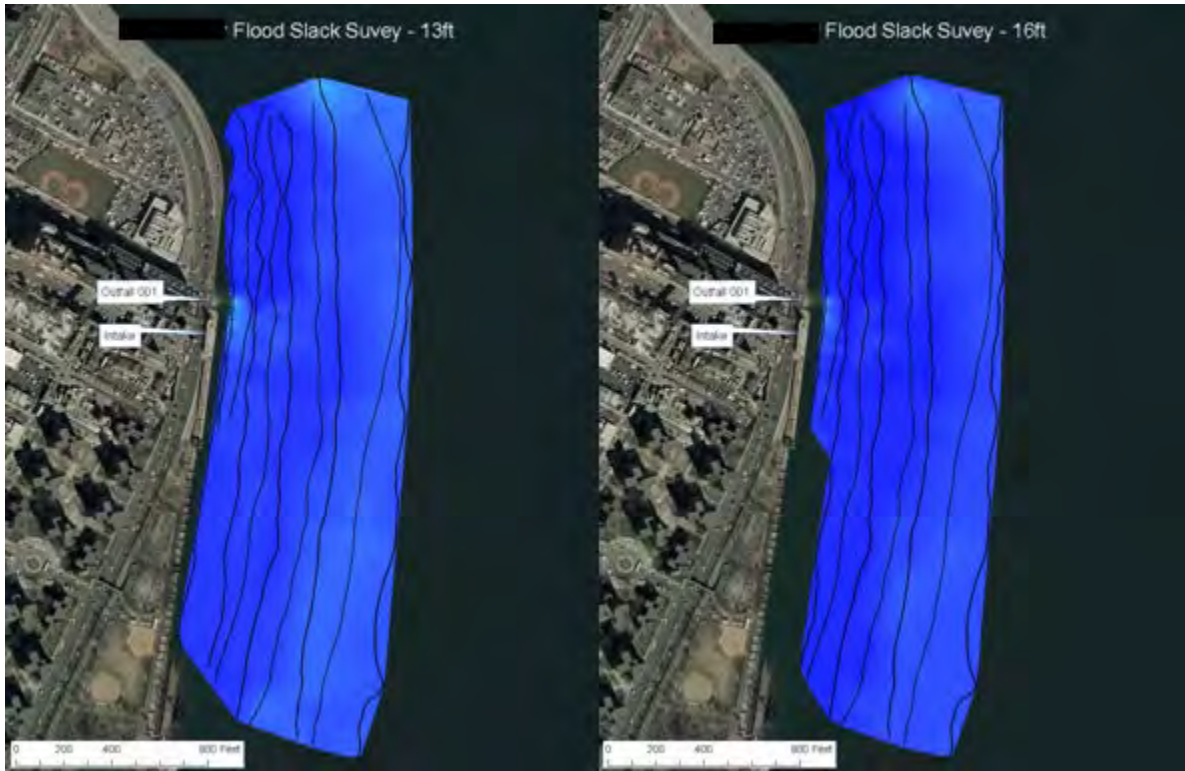
Figure 14-2 (continued) Water temperatures by depth in vicinity of station outfall – flood survey
