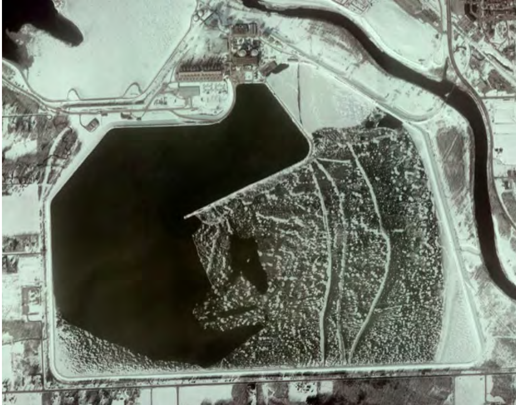
Figure 22-19 Visible photograph of Midland Co-generation Plant cooling lake on February 24, 2008, when lake was partially frozen. Warmer (discharge) side of the lake is not frozen and appears black in this image. Frozen part (intake side) is either pure white (snow on ice) or stippled (uneven ice with ridges).
