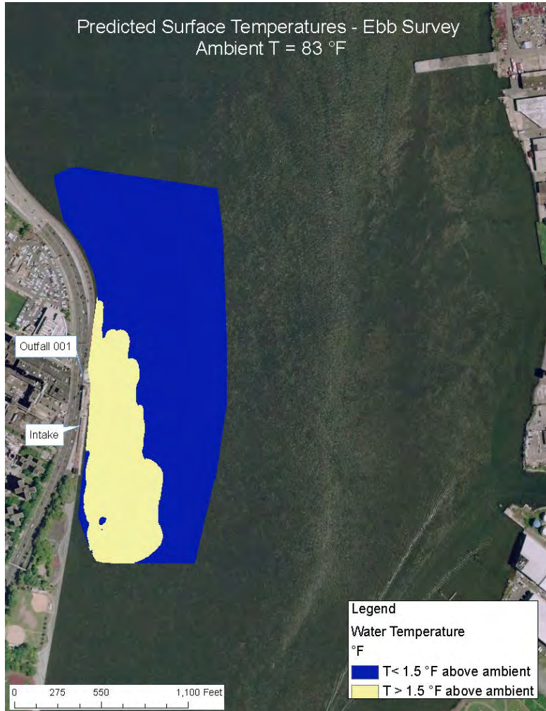
Figure 14-4 Predicted surface temperatures at ebb slack tide in vicinity of station outfall with ambient temperature of 83°F and maximum discharge temperature
