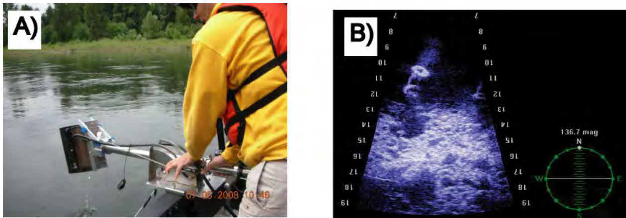
Figure 26-5 Deployment of the acoustic camera. The camera is submerged during operation. Port condition and geometry data from the acoustic camera is used for CorHyd diffuser hydraulic analysis and CORMIX mixing zone prediction.
