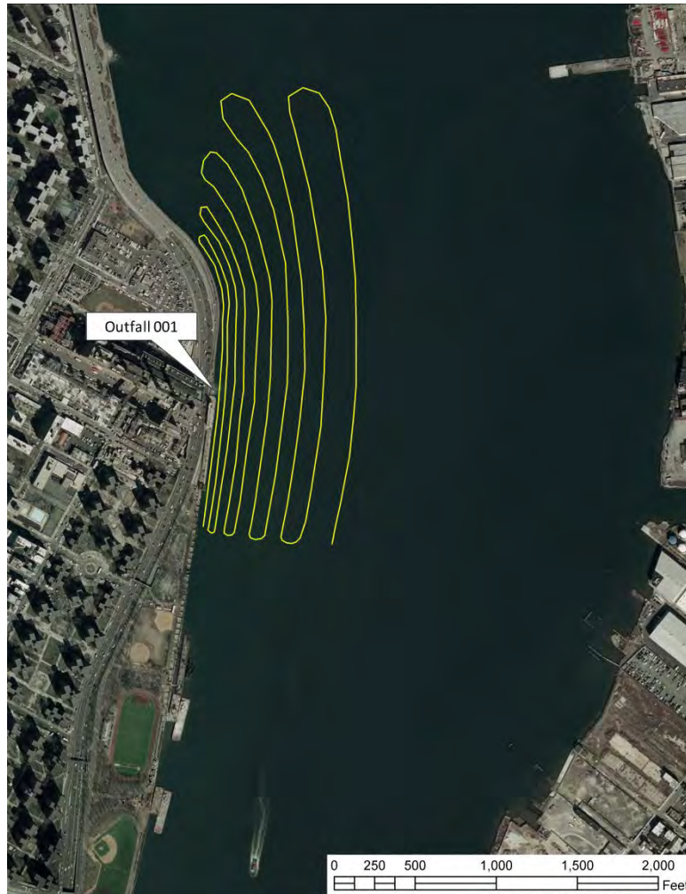
Figure 14-1 Planned temperature survey route in the vicinity of a station outfall. Yellow line shows planned navigation route.
