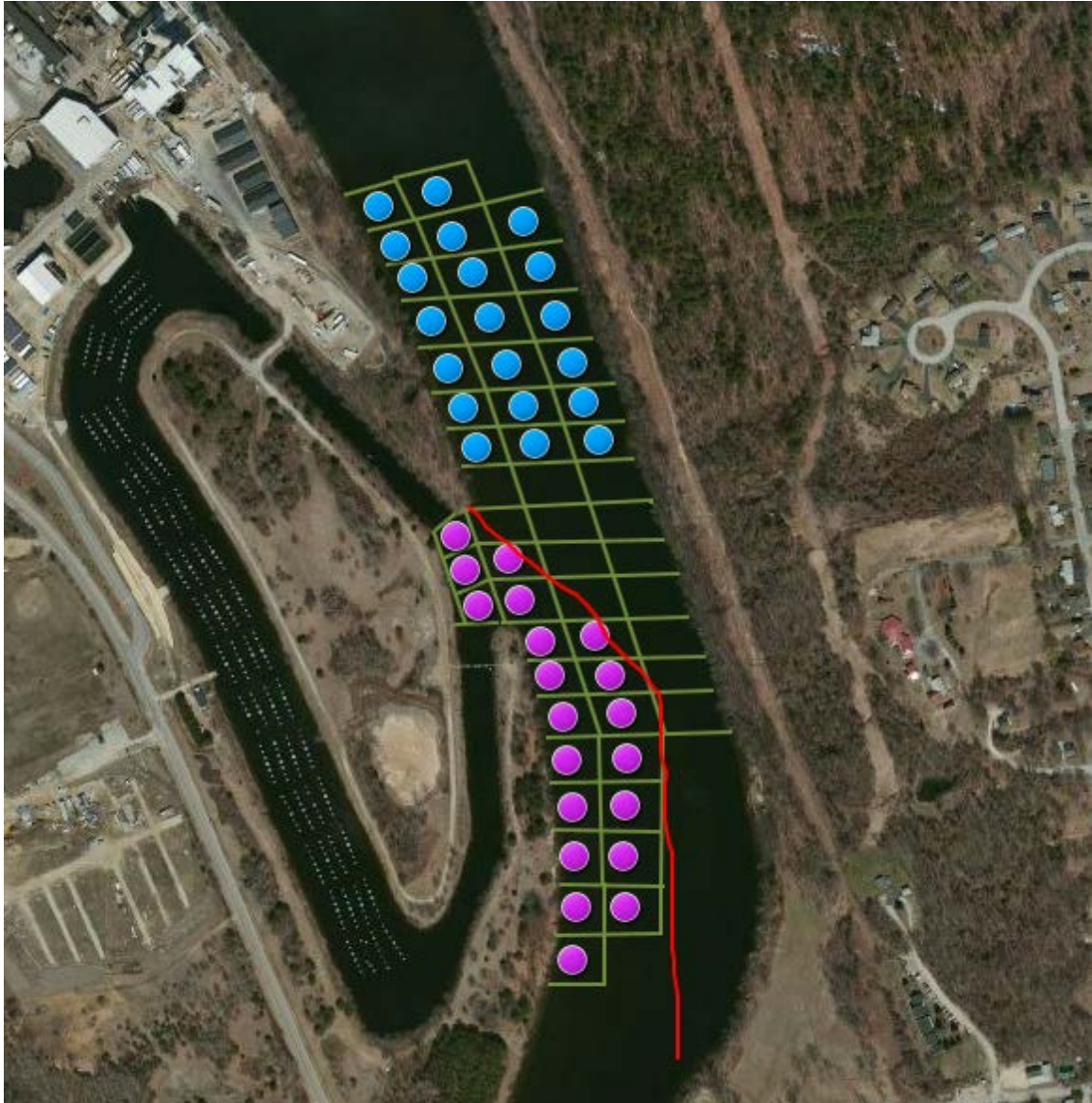
Figure 2: Sampling grid for areas within and outside the thermally-affected zones. Blue dots represent samples within ambient zone, and pink dots are located in the thermally-influenced zone. The red line depicts the approximate limit of ice cover (north and east of) based on an aerial photograph from March 5, 2014.
