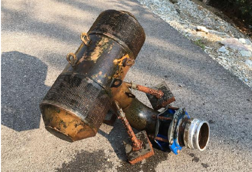
Figure 6 – Post-Test Photo of Entire 12-inch Pilot Test Screen Assembly 3
