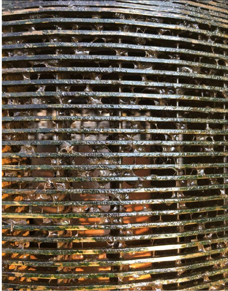
Figure 8 – Post-Test Photo of Downstream Portion of Pilot Test Screen
