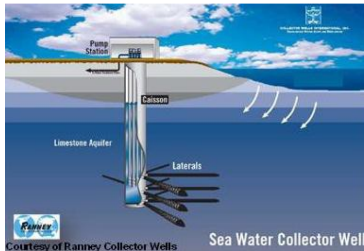
Figure 3-3: Diagram of a radial collector well
