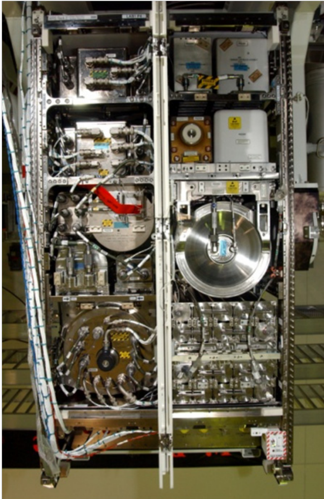
Figure 2 Water recovery system on ISS
