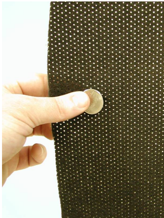
Figure 7-1 Close-up of perforated AFB material (courtesy of Alden)
