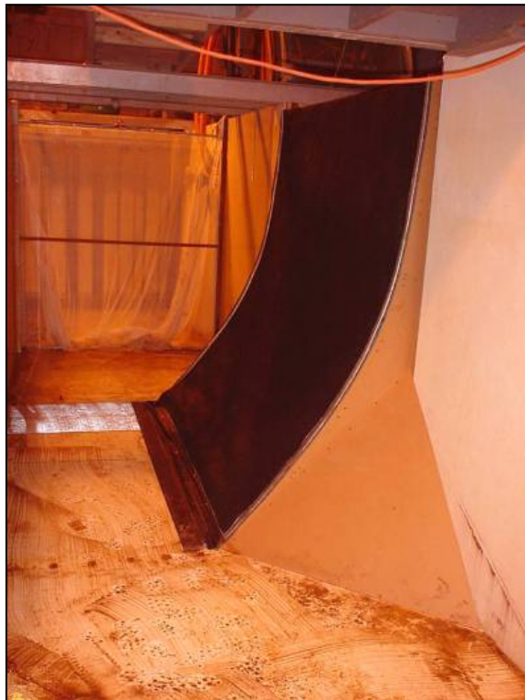
Figure 7-8 Large flume used in the investigation of the effects of ambient sweeping currents on headloss. AFB is installed to simulate the bottom portion of a floating anchored deployment oriented parallel to the ambient flow (EPRI 2004).
