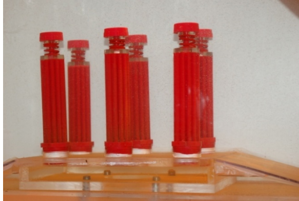
Figure 17-3 Six individual Filtrex filter candles installed in the laboratory test facility.
