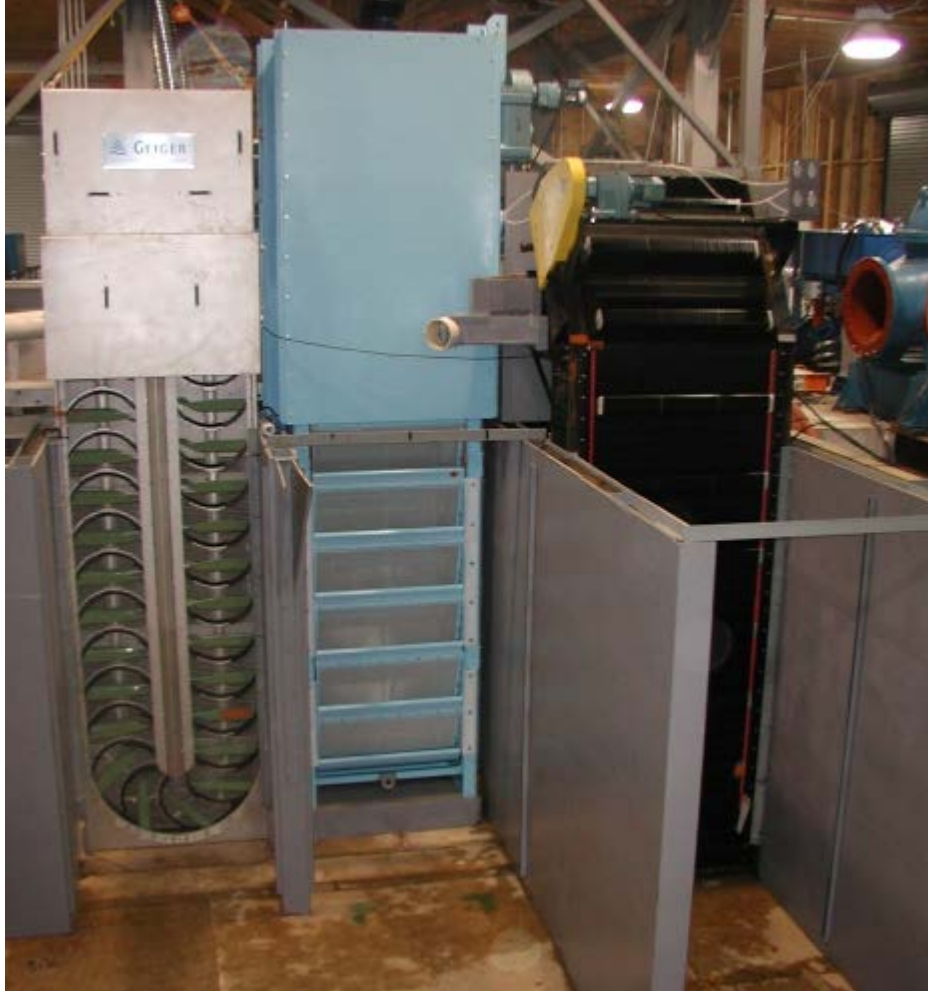
Figure 2-27 Test flume for prototype-scale screen testing showing the three test screens (EPRI 2009b).
