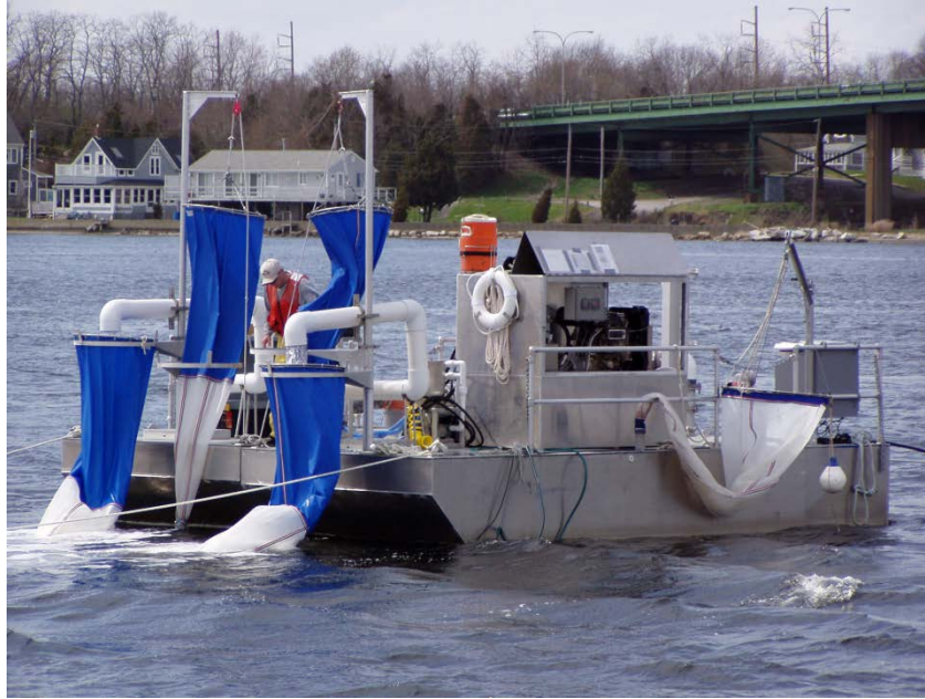
Figure 5-17 Floating test facility (barge with standard sampling equipment) (Alden 2010)
