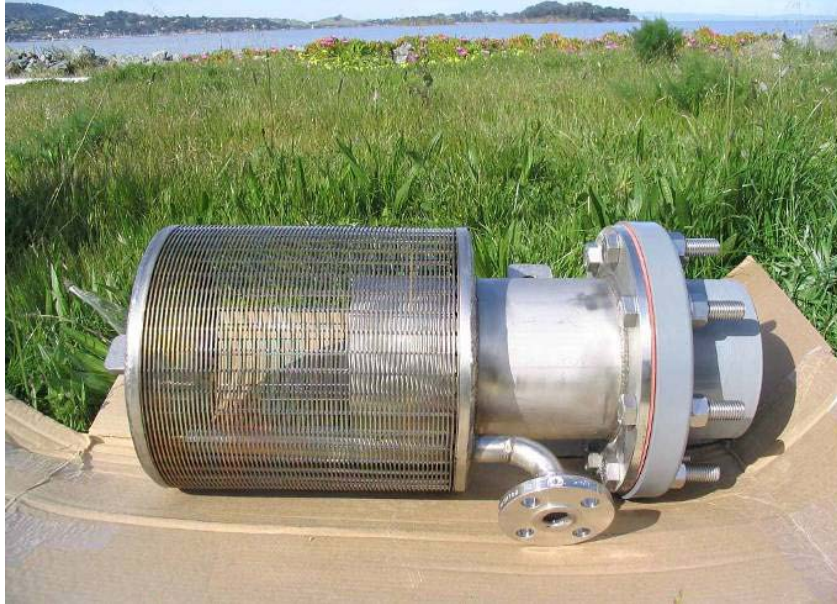
Figure 5-19 MMWD pilot plant cylindrical narrow slot intake
