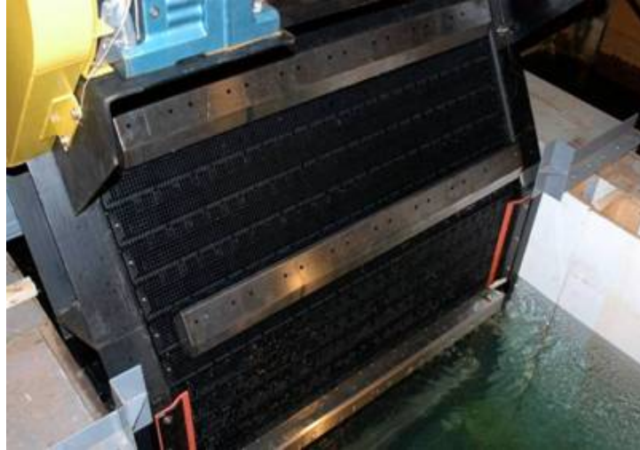
Figure 2-25 Hydrolox Screen™ installed in fish testing flume
