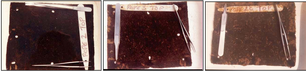
Figure 7-5 Appearance of AFB pieces after 11, 20 and 29 days of exposure (moving from left to right) to water in Bowline Pond at a depth of 3 ft (Henderson et al. 2001).
