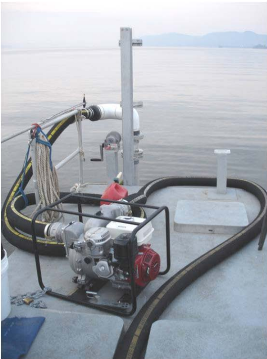
Figure 5-16 Floating test facility (barge) with alternative sampling equipment. Left image show intake side of barge and right image shows discharge side of barge (Alden 2010).
