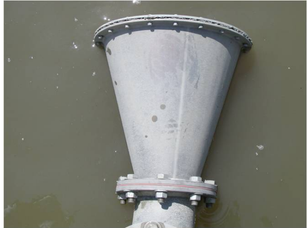
Figure 5-15 Photographs showing the aluminum sleeve used to decrease the open area of the 2.0-mm wedgewire screen (left) and the geometry of the control intake cone (Alden 2010).
