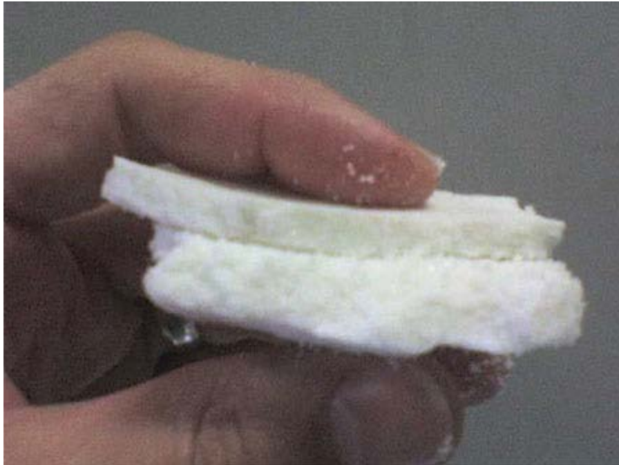
Dry salt generated by the WFGD ZLD System at Torrevaldaliga, Italy. Photo courtesy: Aquatech International.
