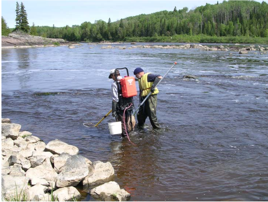
Figure 5. Backpack electrofishers are designed so that the anode (yellow), to which the fish are attracted, is held by the operator, and the cathode (pink) trails behind. Photo by Cam Portt.
