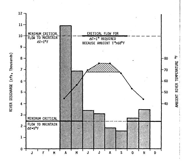
Figure 3. Mean monthly river discharge and ambient water temperature from 1968 to 1977. Merrimack River Thermal Dilution Study, 1978.
