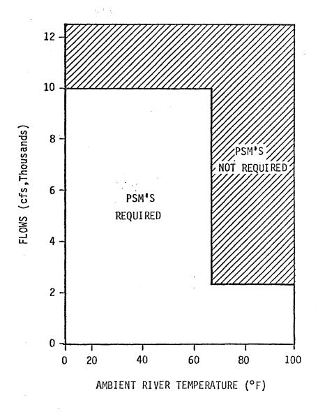
Figure 2. Power spray module (PSM) operation as related ambient temperature and river discharge conditions. Merrimack River Thermal Dilution Study, 1978.
