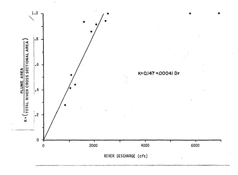
Figure 1. The ratio of thermal plume cross-sectional area to total river cross-sectional area (k) at Station S-4 as a function of river discharge ( $D_R$ ). Merrimack River Thermal Dilution Study, 1978.
