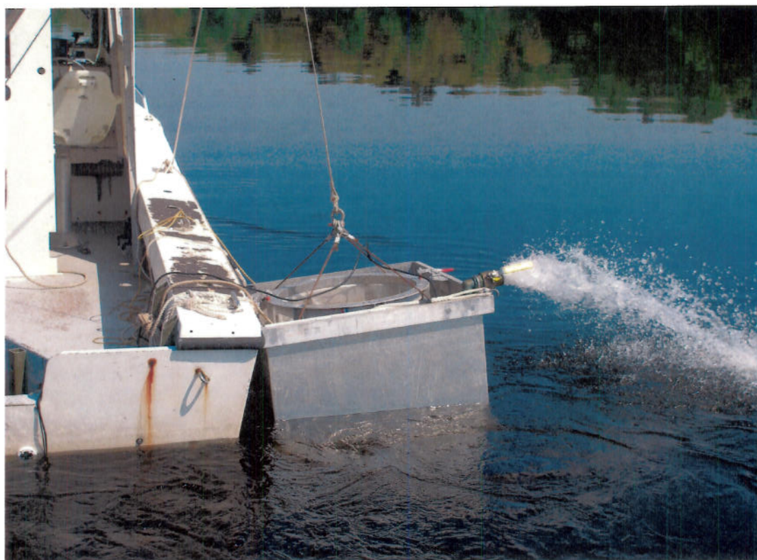
Figure 2-5. Control sampling tank for entrainment survival studies at Merrimack Station.
