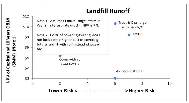
FIGURE 3 Decision Grid - Gypsum Pile Runoff Options
