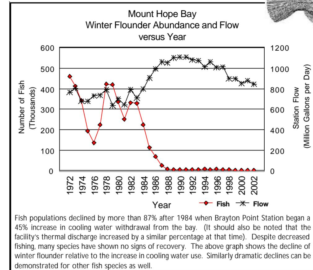
Average annual losses of fish eggs and larvae due to existing cooling water withdrawals at Brayton Point Station include:
