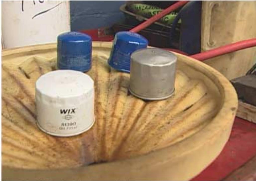
**Oil filters draining into a Collection System**
