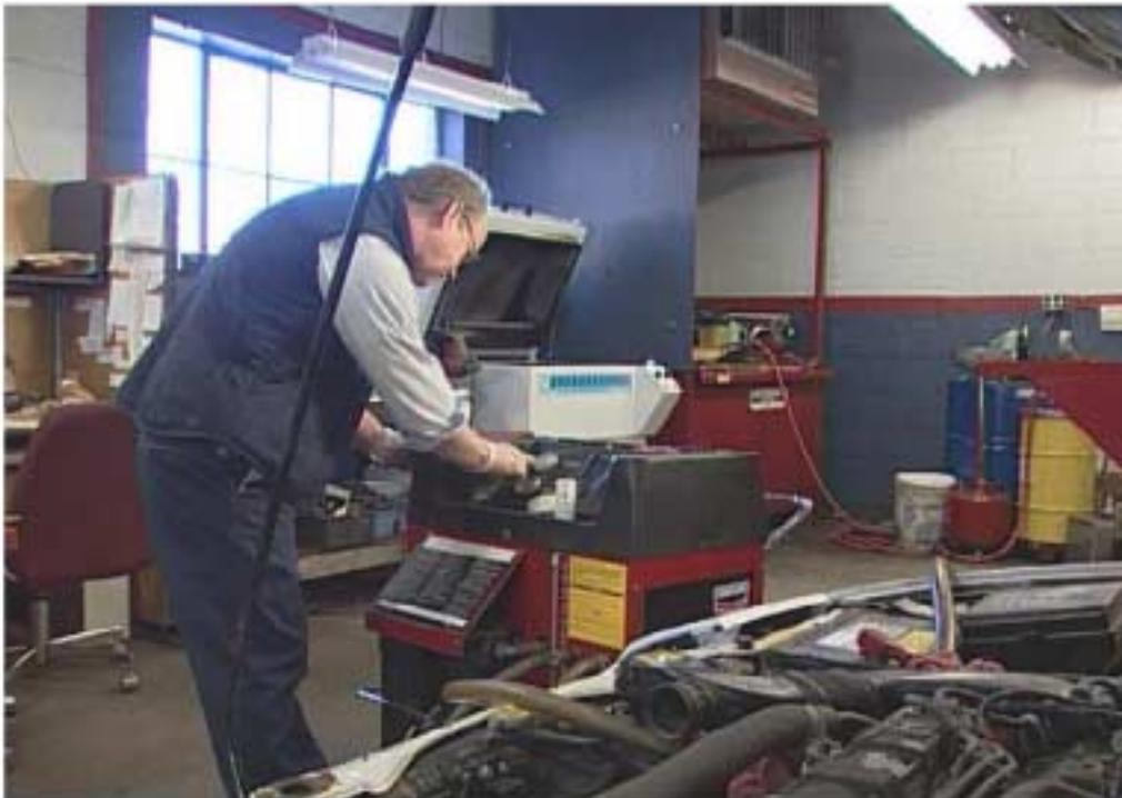
**A Technician tests antifreeze at a mobile pump station that is connected directly to the vehicle's radiator. The antifreeze will be recycled.**
