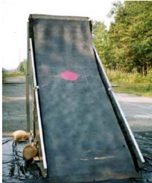
Figure 2-6. Example of Granular Rubber Projectile Containment System (MAARNG 2007a)
