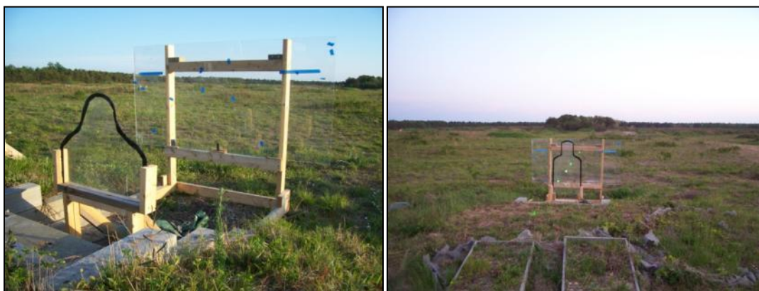
Figure 2. Temporary Plexiglas Targets and Backstops erected at each SIT location to provide a surface to mark laser “impacts” according to a hypothesized target distribution and dispersion patterns.
