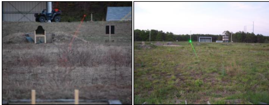
Figure 1. Laser Target Designators: AN/PEQ-15 Advanced Target Pointer Illuminator Aiming Light (Red) and the Beamshot, GreenBeam 2200 GreenBlaster (Green)
