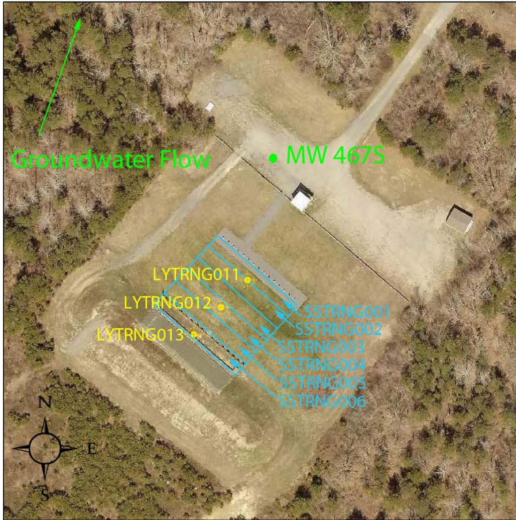
Figure 4. Lysimeters, Soil Grids, and Monitoring Well on Tango Range Camp Edwards, Massachusetts.
