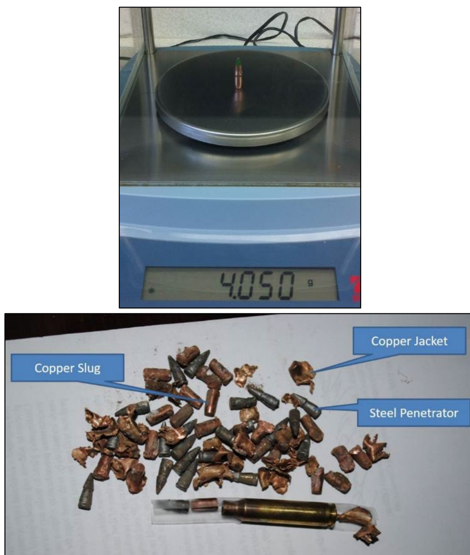
Figure 9. Intact Copper Bullet and Projectile Fragmentation, Camp Edwards, Massachusetts.
