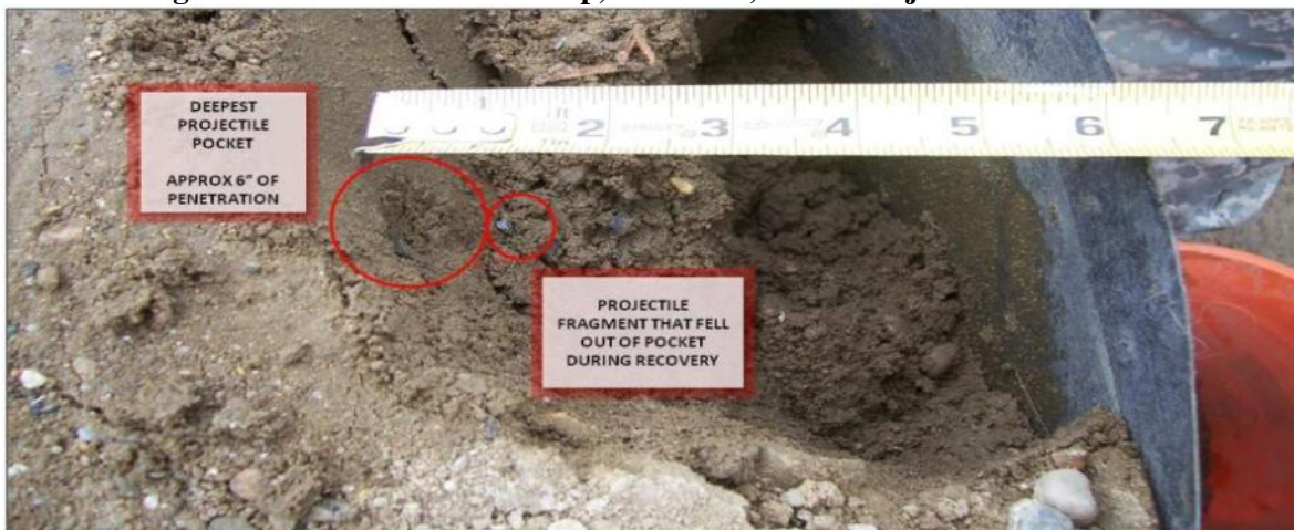
Figure 29. DefenCell® Backstop, 25 meters, 6 inch Projectile Penetration.
