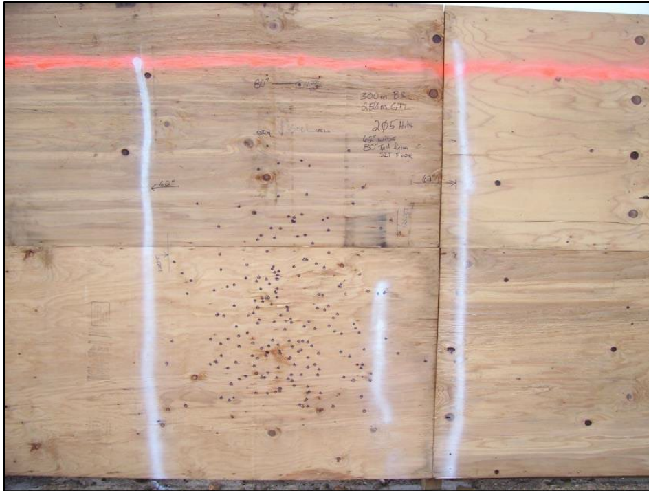
Figure 5. Three Hundred Meter Target Berm Overshot Plywood Telltale after Test Fire Sierra Range, Camp Edwards, Massachusetts
