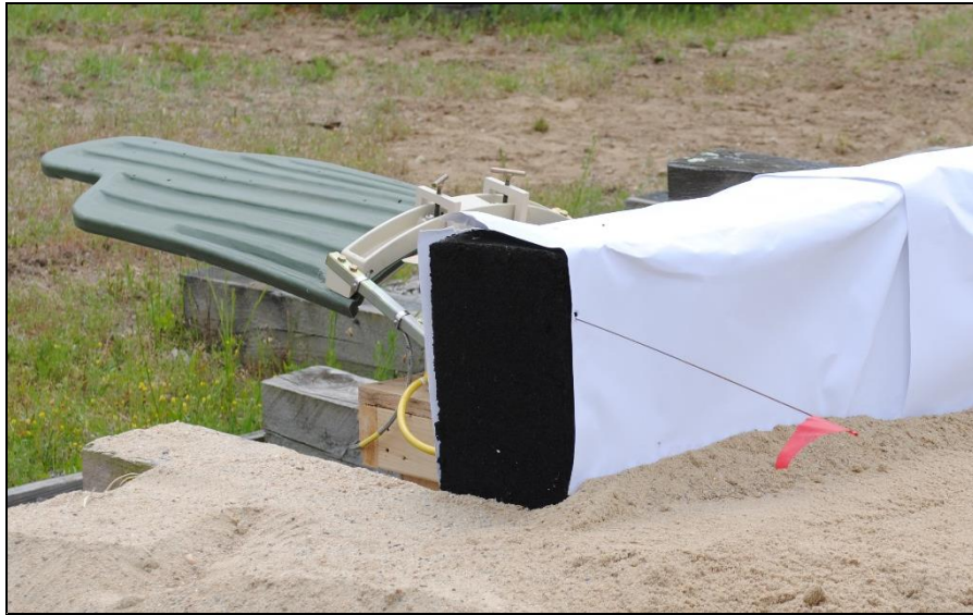
Figure 3. Dura-Bloc on end with flagged projectile pass through, Camp Edwards, Massachusetts
