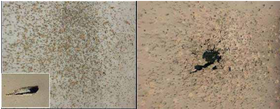
Figure 4-2. Examples of Wear and Deterioration of the Self-Closing Rubber Membrane on the STAPP™ System (photo not taken at Camp Edwards)
