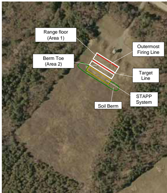
Figure 6-5. Surface Soil Sampling Areas (Area 1 consists of 5 decision units ~ 44x5 meters each; Area 2 is 1 decision Unit ~ 44x5 meters)
