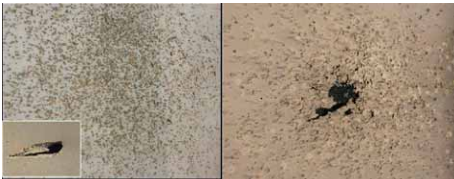
Figure 6-1. Examples of Wear and Deterioration of the Self-Closing Rubber Membrane on the STAPP™ System
