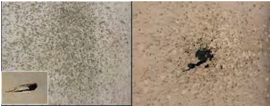
Figure 4-2. Examples of Wear and Deterioration of the Self-Closing Rubber Membrane on the STAPP™ System (photos not taken at Camp Edwards)
