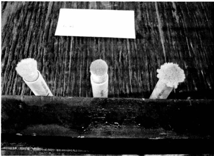
Photograph B-5: Two Negative Samples and Positive Control Sample for Surface Lead.
