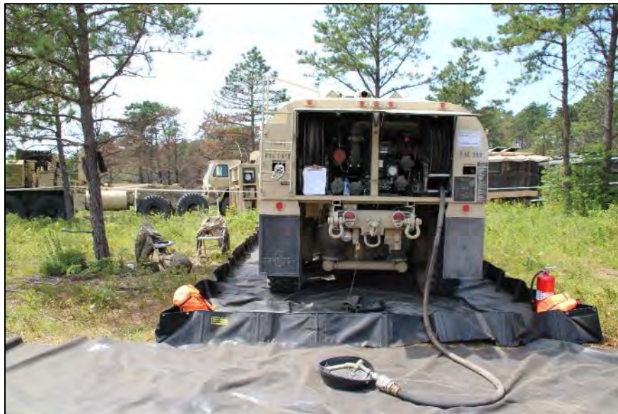
Photograph 2-5 A HEMTT is set up for refueling operations in the Reserve during the CAX. The HEMTT sits on secondary containment to prevent the threat of a spill.
