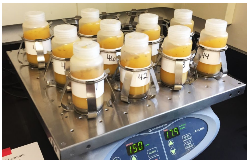
Figure 1. Batch-reaction shaker-table setup, showing reactions 41–50 (iron amendment).
