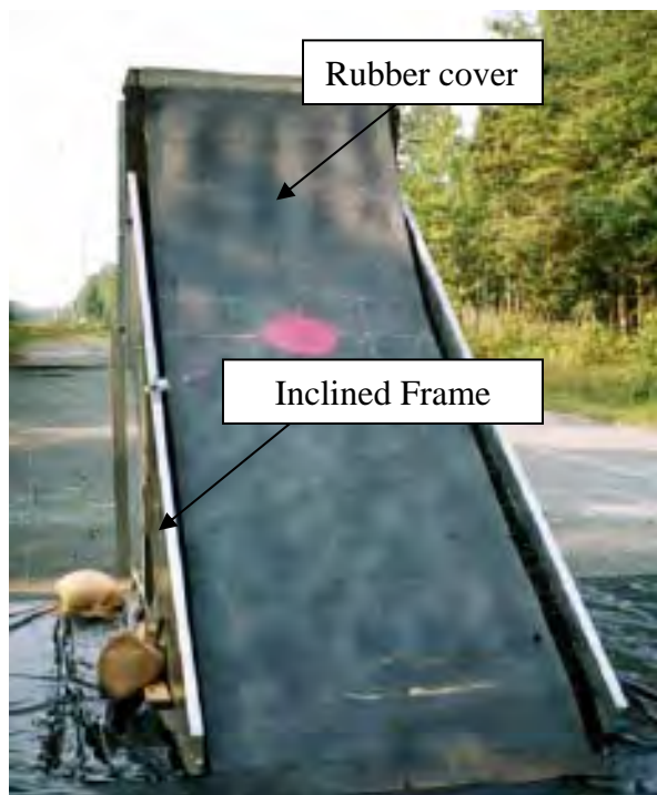
Figure H-2. Granular Rubber Containment System
