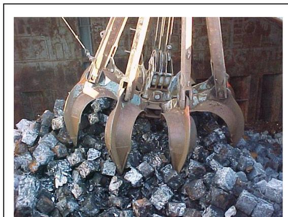
Grapple fitted with radiation detector transferring scrap metal
