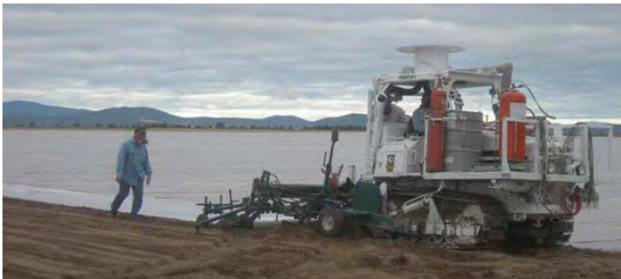
Figure 2-4. Photograph showing flat fume or broadcast shank injection application followed by tarp covering.
