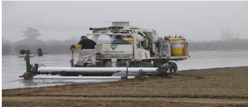
Figure 2-5. Photograph showing shank injection application to raised beds followed by tarp covering.
